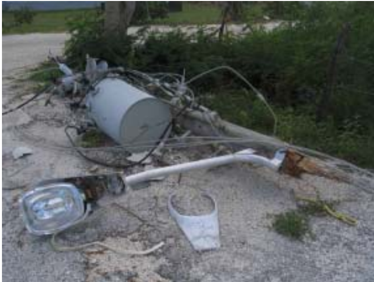
Figure 3.12 Uppermost part of wooden distribution pole broken by wind due to increased total wind pressure (due to higher surface area resisting the wind) and increased gravitational load (weight of the transformer).
