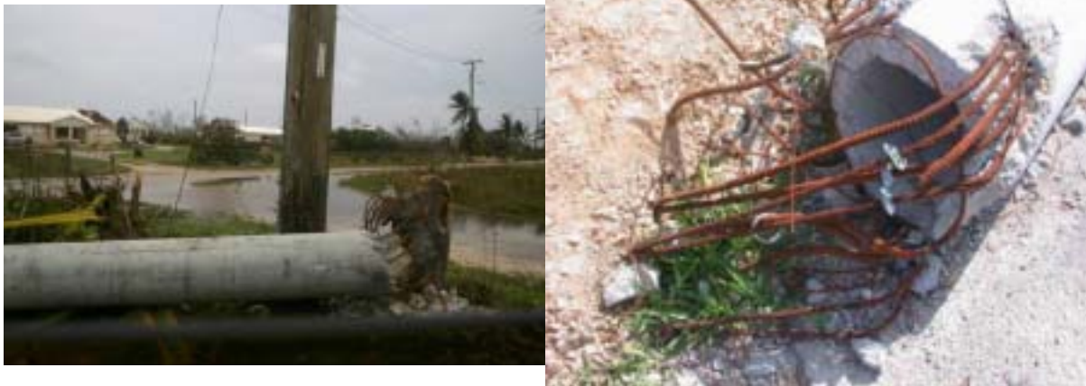
Figure 3.10 Failure of concrete distribution poles in the West Bay area.
